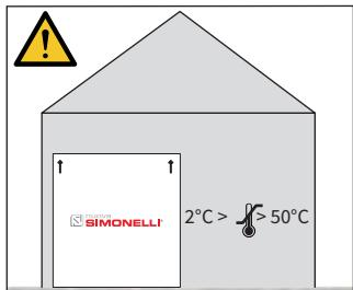
The package containing the machine must be stored away from atmospheric agents. Before performing the following operations, make certain that the load is in stable and will not fall when the straps are cut.
